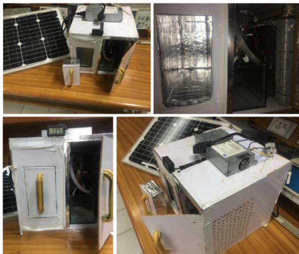
Figure 3: Final Product of Peltier-Based Thermoelectric Cooling Module
