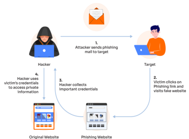
Fig. 1. Phishing attack process [1].
