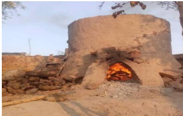
Fig. 2. Kiln Firing of Composite Filters.
