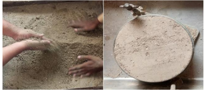
Fig. 5. Soil mixing and finishing (compaction test)
