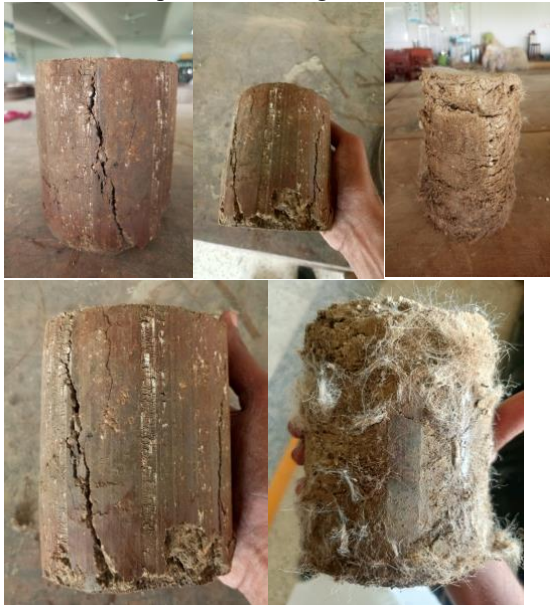
Fig. 11. Failure patterns of different stabilized soil samples (UCS tests)
