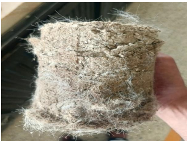
Fig. 12. Failure pattern of combined optimal stabilized soil sample with 1% \text{CaCl}_2 and 0.5% PP fibre
