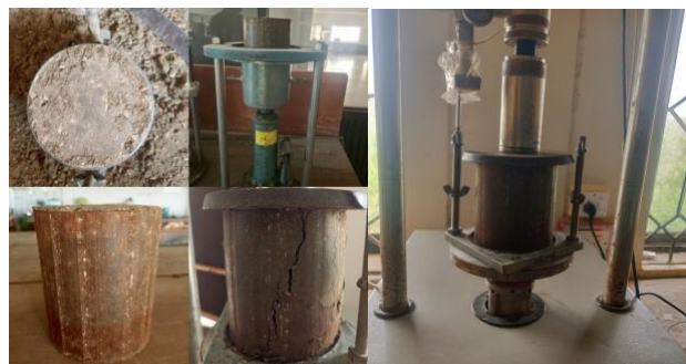
Fig. 7. Steps involved in UCS test
