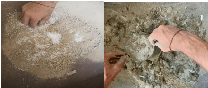
Fig. 3. Soil improvement using \text{CaCl}_2 and PP fibre.
