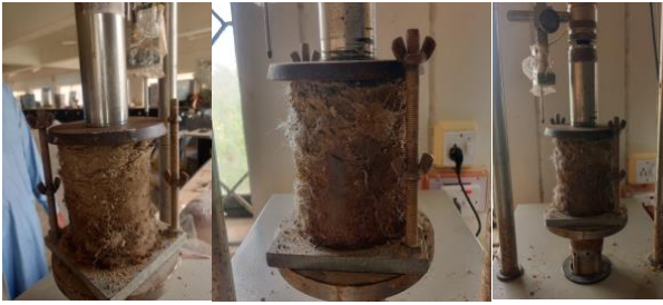
Fig. 8. Unconfined compressive load application
