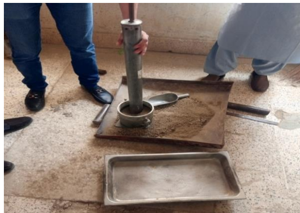
Fig. 6. Soil compaction in layers
